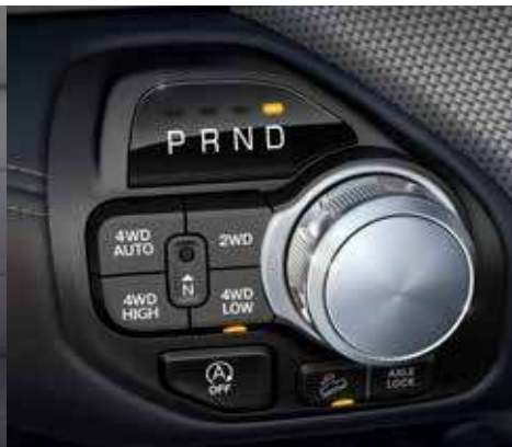
ELECTRONIC SHIFT-ON-DEMAND TRANSFER CASE
